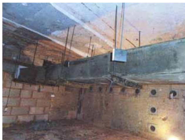
Horizontal duct inside the furnace after the fire test (184 minutes).
