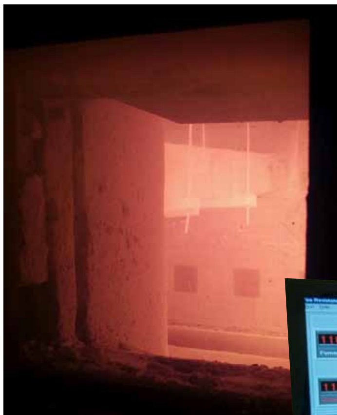
Kemwell horizontal service duct during a fire resistance test to BS EN 1366-5:2010.
